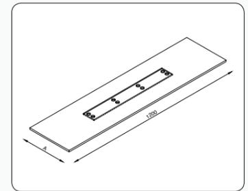
\*When installed with the Wall Grill, the Drainage Component width is reduced by 80mm, to 220mm.
