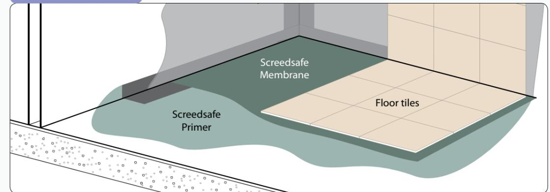
**RIW** Screedsafe is a self-adhesive waterproof membrane designed for use prior to the application of ceramic tiles, and natural stone onto concrete and screeded in wetrooms and other critical areas.
