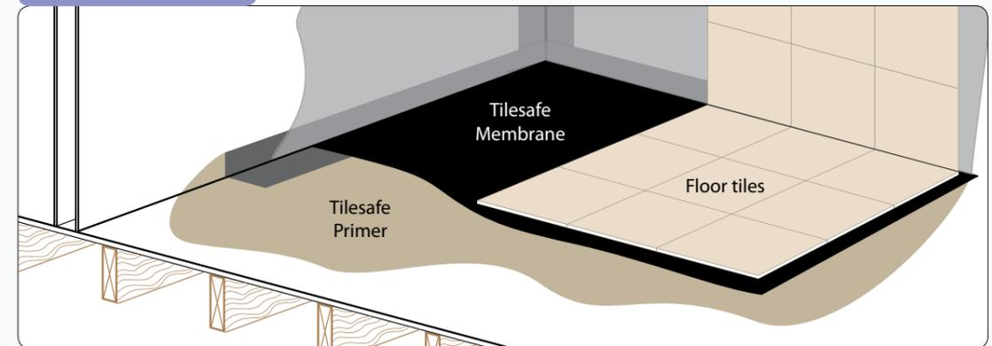
**RIW** Tilesafe is a self-adhesive waterproof membrane designed for use prior to the application of ceramic tiles and natural stone onto timber and solid floors in wetrooms and other critical areas.
