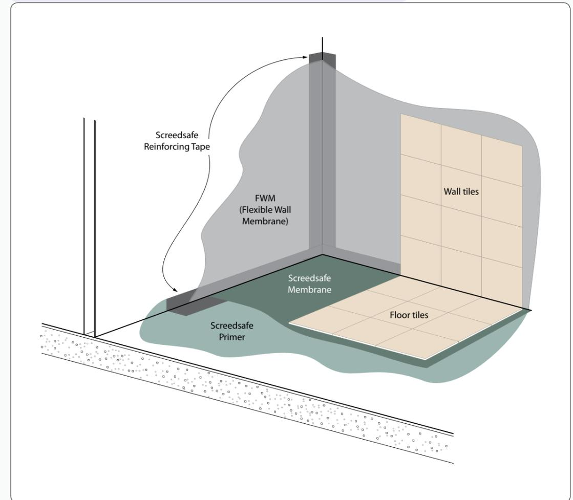
**For solid floors** we recommend that the Screedsafe membrane is applied to the shower area plus an additional one metre in either direction.
