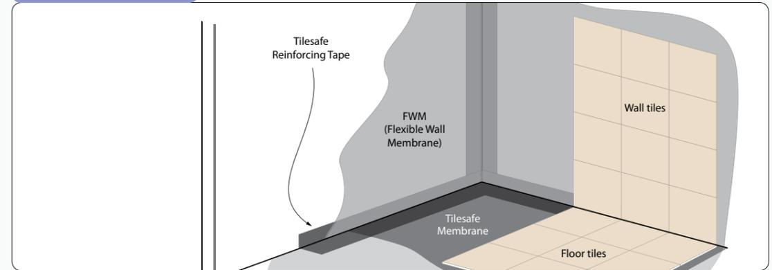
**RIW** FWM - Flexible Wall Membrane is a flexible coating for waterproofing wall surfaces prior to the application of ceramic tiles and natural stone in wetroom and other critical areas.
