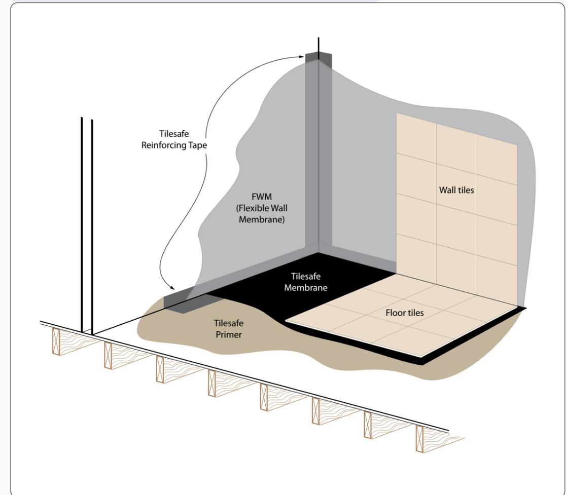
**For timber floors** we recommend that the Tilesafe membrane is applied to the entire wetroom floor.
