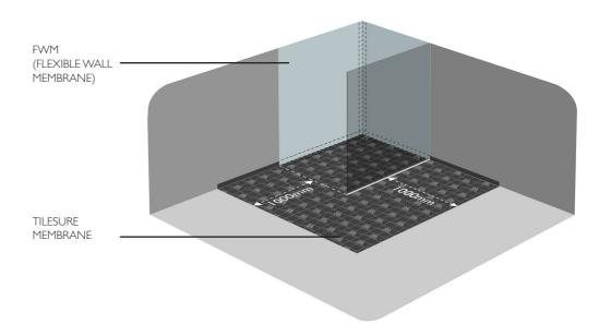
For larger bathrooms or where cost may be a consideration, Tilesure should be applied to a minimum of the shower area, plus an additional one metre in all directions. FWM <sup>‡1</sup> should be applied to the walls within the shower area only, to a minimum height of 2000mm and overlapping the Tilesure Reinforcing Tape.
