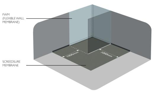
For larger bathrooms or where cost may be a consideration, Screedsure should be applied to a minimum of the shower area, plus an additional one metre in all directions. FWM  $^{\ddagger 1}$  should be applied to the walls within the shower area only, to a minimum height of 2200mm and overlapping the Screedsure Reinforcing Tape.
