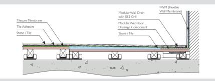
drainage gradient without the need for pouring screed to falls, Linear Screed Decs and infill panels were installed onto the solid floors.
